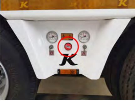
Park freni kontrol paneli
